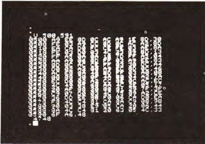
F A typical screen dump showing the squashed display. The Hex pair on the right is the checksum.
